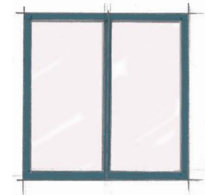
Drop sill with vertical divides.
